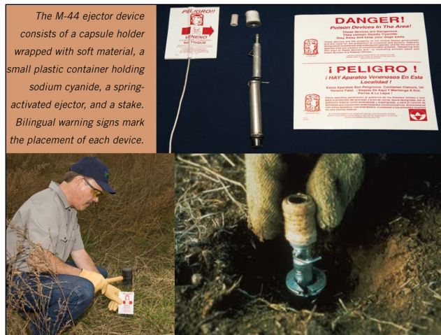
Figure 2. M-44 explosive poison (sodium cyanide) delivery device for killing wildlife (Factsheet May 2010, US Department of Agriculture Wildlife Services; http://1.usa.gov/281v69N ).
